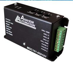
The MDC151-05010 driver is designed to drive DC Brushless Motors at currents of up to 10A (peak) and 50V. Using hall sensor feedback, a constant velocity mode can be selected. The driver is protected against over current (cycle-by-cycle), hall sensor error and under voltage. When an error occurs, a fault light is turned on to notify the user.
